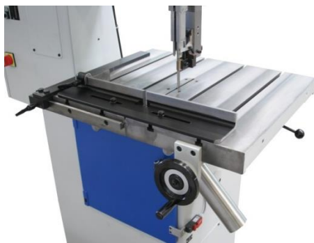
Manual feed table SSF 420, with lead screw
