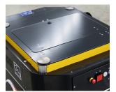
The lifting unit developed by Mössner makes it possible to lift loads and goods by up to 60 mm. This gives the AMR a broader range of applications and extends its field of tasks.
