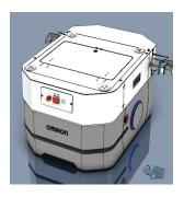
By using two additional laser scanners, the AMR's field of view is increased in height. This results in improved safety for people and enhanced collision avoidance.
