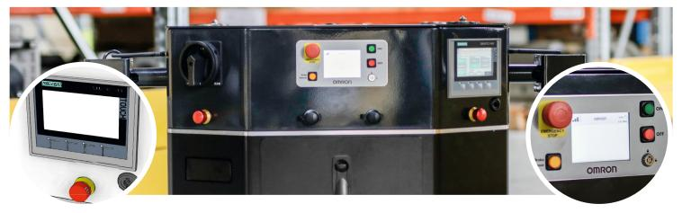
The built in PLC with integrated HMI serves as the interface between the AMR and the lifting unit. The HMI enables manual access to the AMR's control to execute functions directly on the AMR.
